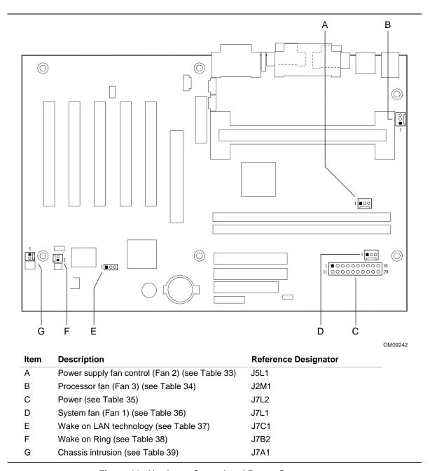
Figure 11. Hardware Control and Power Connectors
